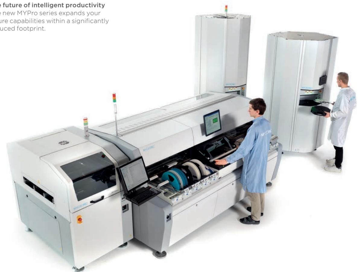
0.15 mm pitch. Both options provide extremely precise on-the-fly positioning and inspection for any type of miniaturized or specialized component.
